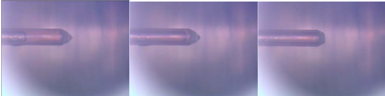
Figure 129. Images showing an air bubble travelling through the emitter and disrupting the spray
