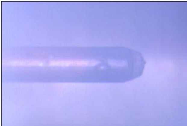
Figure 133. Electrostatic spray formed in a Silica emitter
