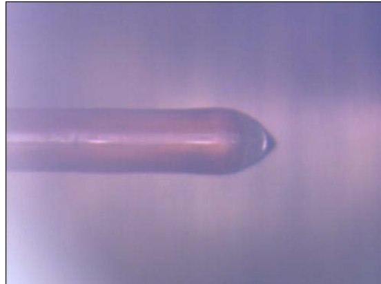
Figure 131. Electro-spray formed in an externally-wet Silica emitter
