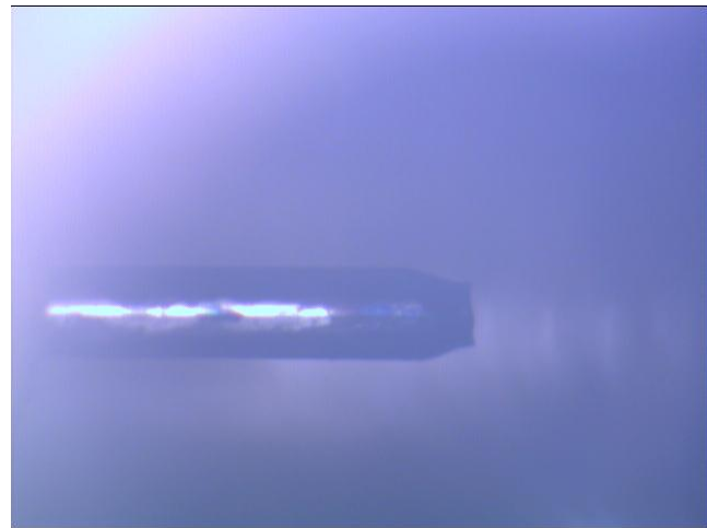
Figure 135. Electro-spray formed in a metallic emitter
