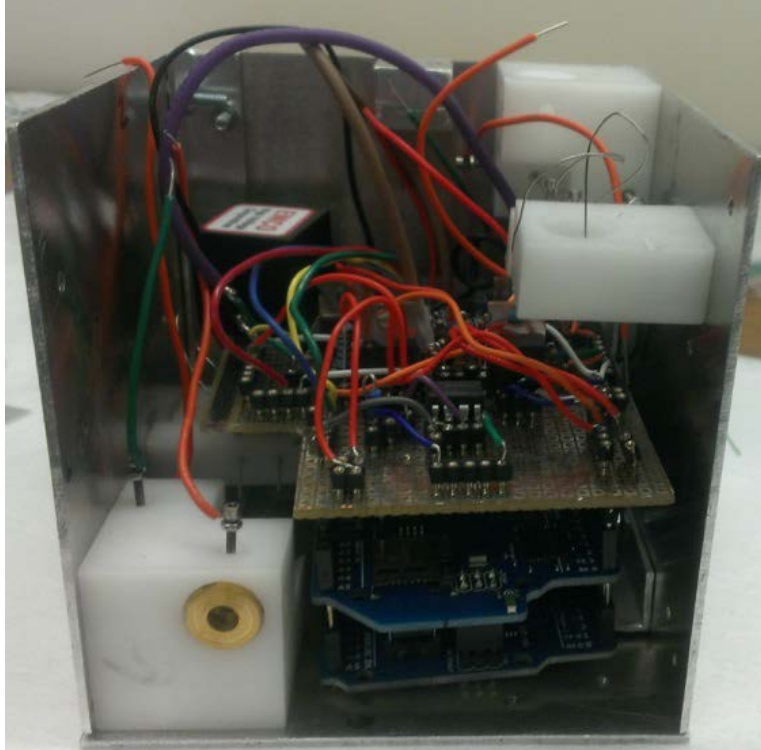
Figure 121. Arduino and the WiFi Shield assembled inside the cube with the two thruster systems
