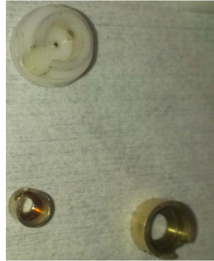
Figure 128. Oxidized internal extractor
